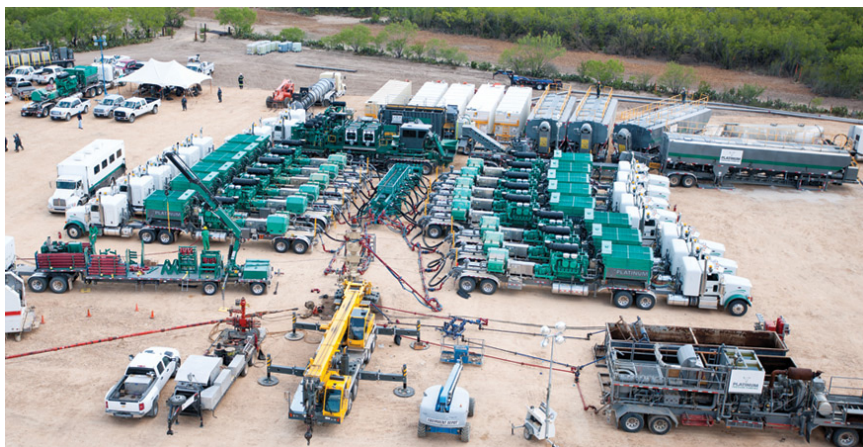
FIGURE 2-5 Photograph of hydraulic fracturing operation in the Eagle Ford Shale. The green trucks are pumps for hydraulic fracturing. Behind them are containers with water, sand, and other materials used for hydraulic fracturing. A wellhead tree appears in front of the pump truck array and behind a yellow crane. SOURCE: Image courtesy of Yantis Company.
